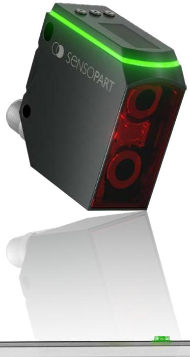
The intuitive operation of the DTECT® Object 3D is supported by a color display on the device. The field of view or the relevant height can be adapted to the application quickly and easily using the appropriate buttons – all without external software. After the teach-in, the operational state or the sensor result of „Pass / Fail“ is visualized by the illuminated frame that is visible from all sides. Further adjustments can also be made easily and intuitively using the IO-Link interface.
