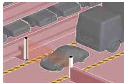
Detection of overall dimensional limits of vehicles in automated parking garages
