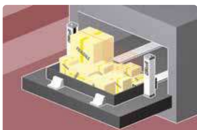
Automatic warehouses: detection of maximum height of the objects present in the tray for efficient management of the machine's capacity
