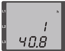
Fig. Operating hours meter display (measuring display A20), example 140.8 h
