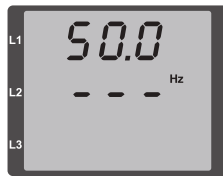
Fig. No direction of the rotary field can be determined ("---").
