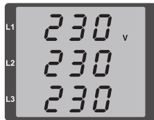
Fig. Example display: Mains voltage per phase
