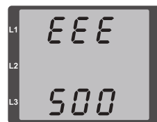
Fig. Error 500 (mains frequency)
