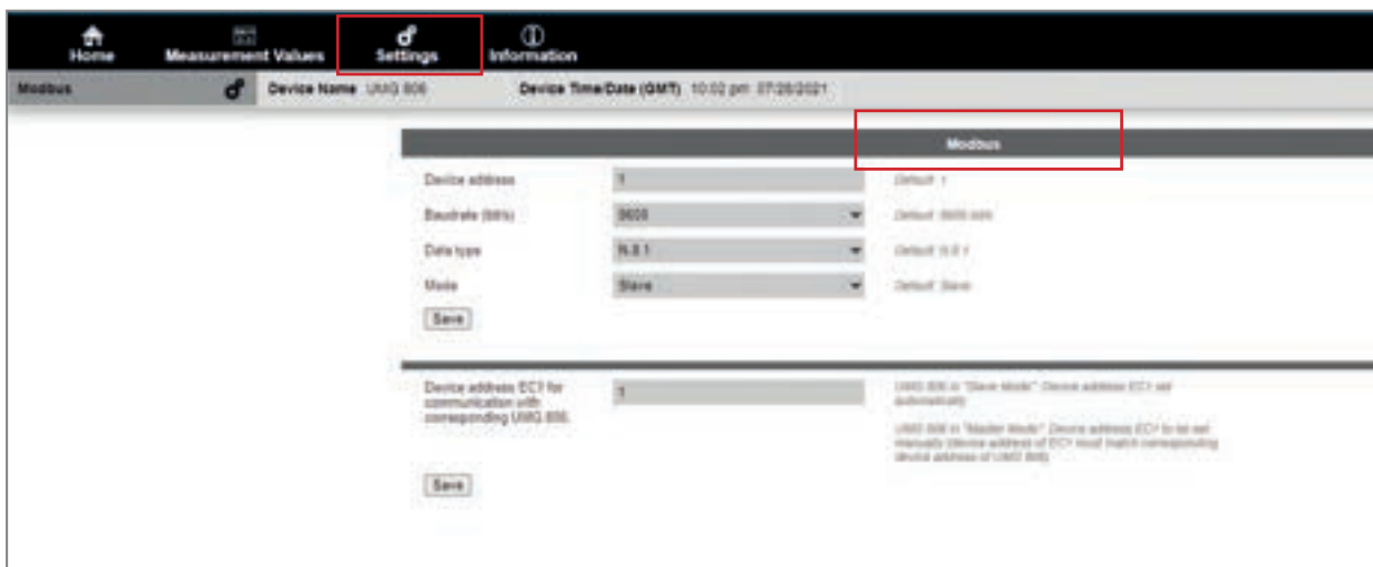
Fig. Example of Modbus settings for the UMG 806 device
