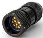
Cable-connecting socket, long housing, 10 pole to VG96934 version J for connection and interconnection cables, available with 5-coding layers and solder terminals up to AWG20
